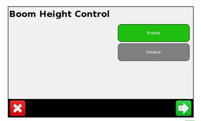
6. In the Welcome to Boom Height Control Setup screen, tap to start the Boom Height Control Setup Wizard.
