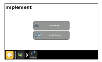
The *Implement* screen contains two options, *Advanced* and *Initial Setup*. The *Advanced* option appears only after you have set up your controller using the *Initial Setup* option.
