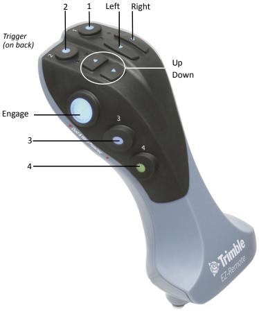
**Note:** The Up, Down, and Trigger buttons are not supported.
