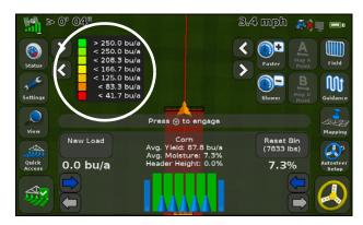
• You can use the grain *Bin* level status item to track the amount of grain in the Grain Bin. Set up the size of the grain bin in the Yield Monitoring Setup wizard. Tap the button to reset the counter:
