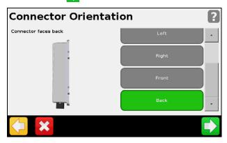
2. In the Label Orientation screen, orient the controller image in reference to the mounting direction of the NavController II Labeling Panel when this is viewed from above, and with the front of the tractor pointing to the top of the display. Ignore the reference direction of the Nav II wiring connectors during this step. When the correct connector orientation has been achieved, tap 💎
