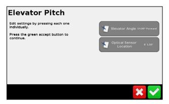
**Note** – Failure to set the correct optical sensor spacing from the rear wall can cause degraded performance.
