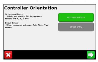
Controller Orientation is set by using Orthogonal Entry or Direct Entry—tap when you have made your selection in this screen and then follow the procedures described below.
