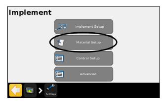
2. In the Material Setup screen, tap New Material.
