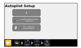
**Note** – The buttons that appear depend on the vehicle loaded from the vehicle database (VDB) or from a restored vehicle configuration. The following is a complete list of what may appear—some or all may be relevant to your selected vehicle type.
