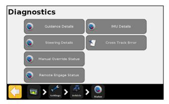
In the *Diagnostics* screen you can view the main sensor inputs for the selected vehicle type. The raw and scaled sensor data values will appear on each page. Data in the *Diagnostics* screen is updated continuously to allow for real-time evaluation of the connection.
