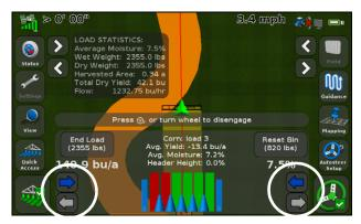
• Tap **New Load** to start and stop loads for calibrations and load tracking. The CFX-750 display can hold up to 250 loads:
